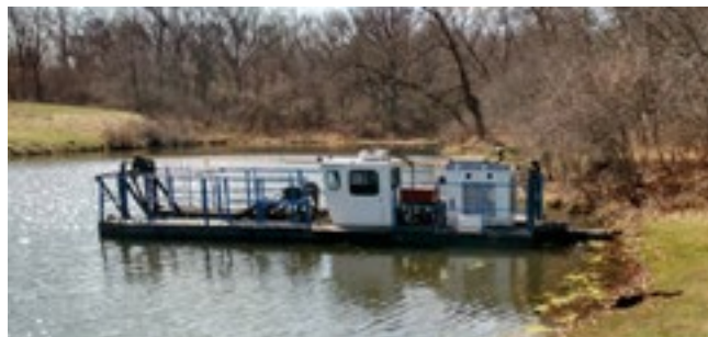
Dredge launched into Hidden Lake on March 26 in preparation for dredging. The dredge is approximately 30 feet long.
